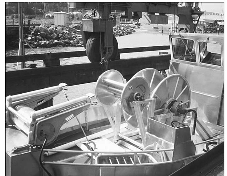
**TAKING UP** most of the Chris K's deck space is net hauling equipment: a power roller, herring shaker and sliding net reel.
