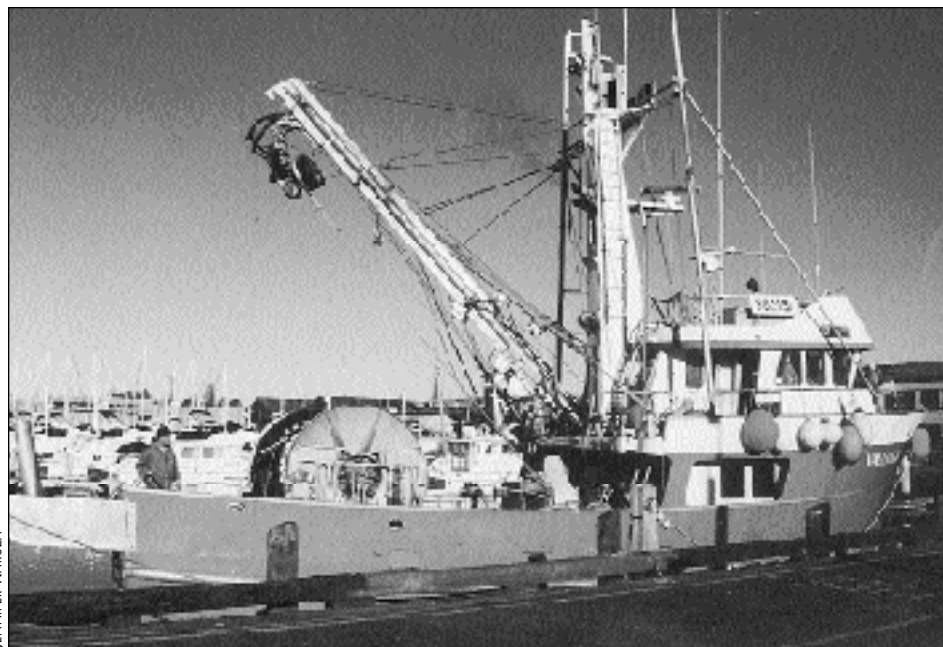
THE SECOND EDITION of the Valiant Lady, an aluminum 58-foot Alaska seiner, was inspired by Canadian vessels but launched in 1991 from an Alabama boatyard.
