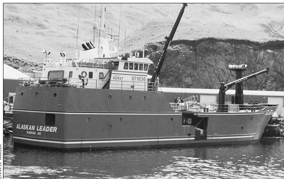
THE 150-FOOT Alaskan Leader was the first freezer-longliner of Delaney's original partnership. Built in 1990, it was the largest such U.S. vessel ever constructed.
